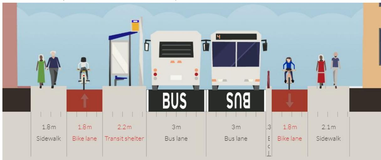
Here, we have proposed a 2.2 m wide island bus stop. We do not believe this is excessively narrow for an urban village. In Copenhagen, there is a comparable road to Rathmines Road, which has recently had a bus gate installed. In order to fit in bus stop bypasses, they have used island bus stops even narrower than those proposed above (~1.6 m), and they have created a chicane between the opposite direction stops to minimise wasted space.
