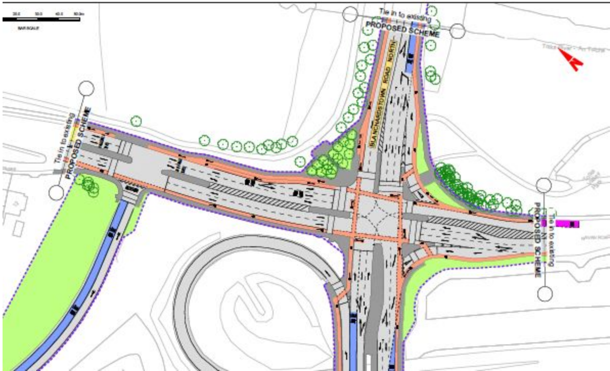
Figure 3 Illustrating Slip Lanes (Blanchardstown Rd Junction) Cutting Across Cycle Lanes Against National Cycling Manual Recommendations
