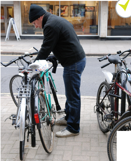
Fig. 1 Stands 1000mm apart allow cyclists to lock their frames in comfort
