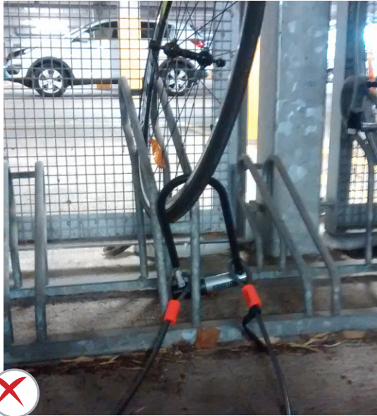
Fig. 14 Wheel racks allow the quick release wheel to be undone and the rest of the bike to be taken
