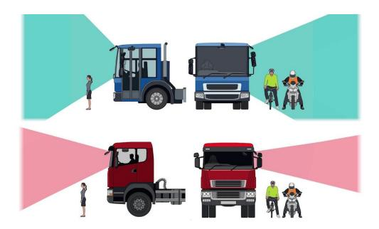
Transport for London (TfL) has set <u>direct vision standards (DVS)</u> for all HGVs entering London. Direct vision standards assess how much a driver can see directly from their HGV cab. This is the solution to "blind-spot" issues that lead to the deaths of cyclists and pedestrians near HGVs.
