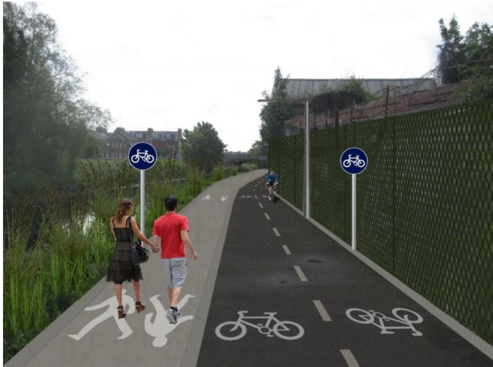
A photo-montage of the Royal Canal Greenway with segregated space between pedestrians and cyclists. There is a curb separating the cyclists from the pedestrians.
