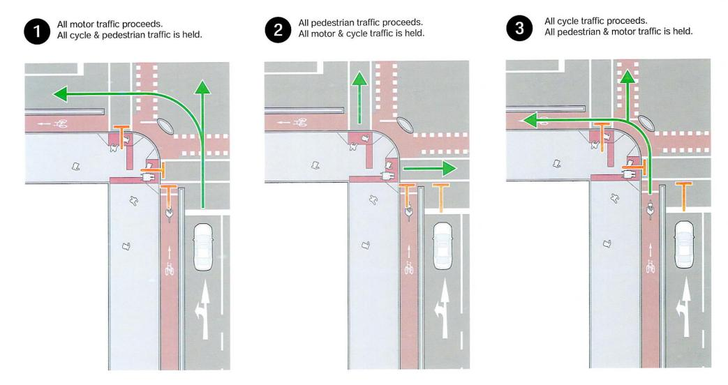
NOTE: Interupting the cycle lane with the controlled pedestrian crossing will add an extra 5m to the pedestrian crossing span.
