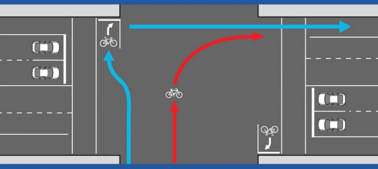
INSTEAD OF BEING IN THE CENTRE OF THE ROAD (RED ROUTE) FOR RIGHT TURNS, USE THE TWO-STAGE 'HOOK TURN' (BLUE ROUTE) TO KEEP OUT OF DANGER.
