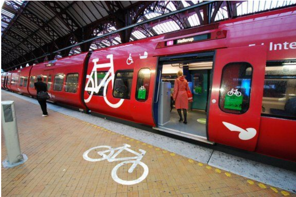
Carriages and platform marked to give passengers an indication where bike storage will be on the metro vehicle
