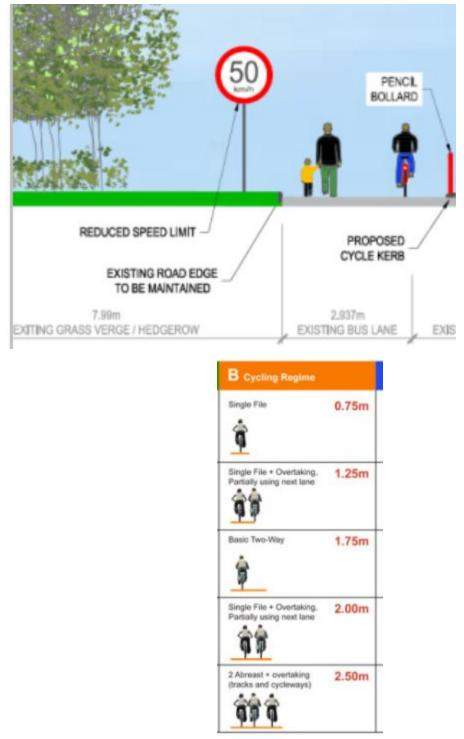
While the drawings are not detailed, they mention a typical layout will be a 1.85m footpath next to a 1.85m cycle lane with a kerb and possibly bollards. The footway and cycle track look flush which is not good for pedestrians - the footway should be higher than the cycle track so that
