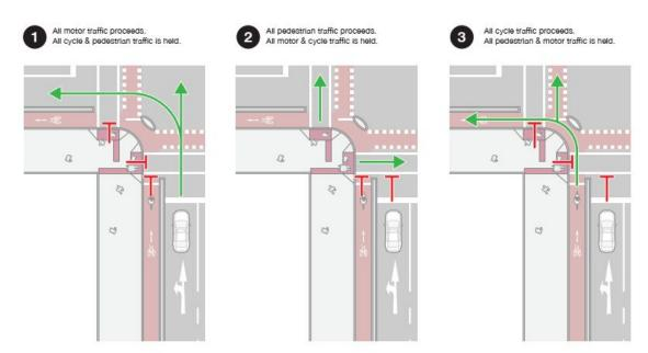
NOTE: Interupting the cycle lane with the controlled pedestrian crossing will add an extra 5m to the pedestrian crossing span.
